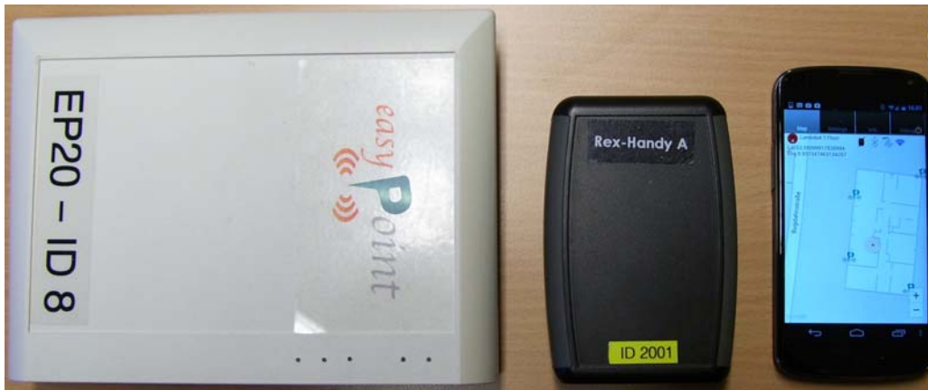
Figure 4: Hardware prototypes anchor node "easyPoint", tag "Rex" and mobile device with indoor localization app
